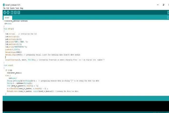
Figure 2: Sample Code for Forming and Sending Sensors Data from Nodeto the Main Node.
